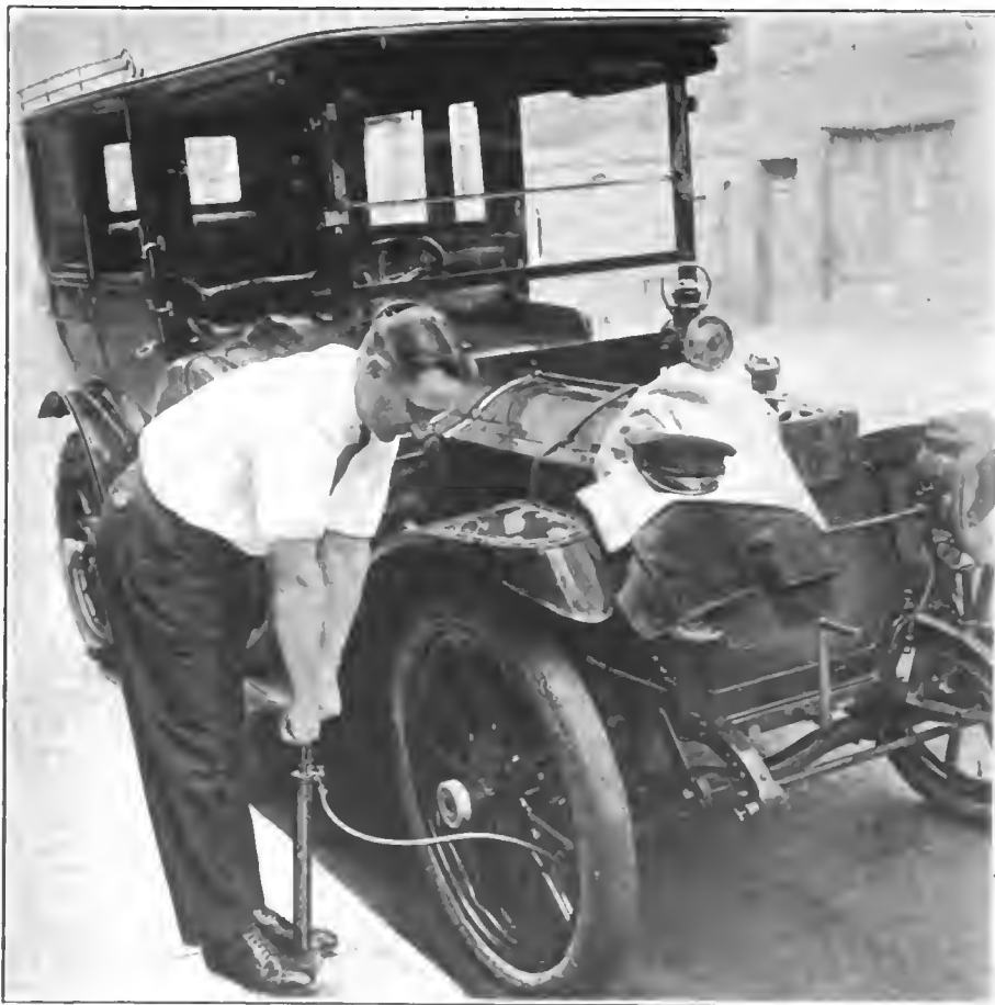
Fig. 1—Inflating big tires with a small hand pump—no chance of the pressure being enough to prevent flexure—the unfortunate pumper is really working hard to increase tire depreciation whether or not it is agreeable to him.
